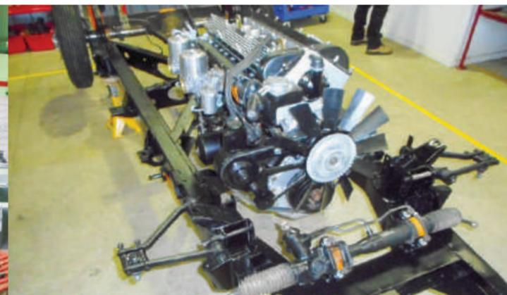
Images showing the MkV donor chassis being prepared for modification and painting; one of a series of line drawings illustrating various body style options; and the fully rebuilt 4.2 litre XK engine installed in the immaculate chassis, along with some suspension pieces and the steering.
