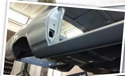
Replacement of rusted-out metal has already begun.
