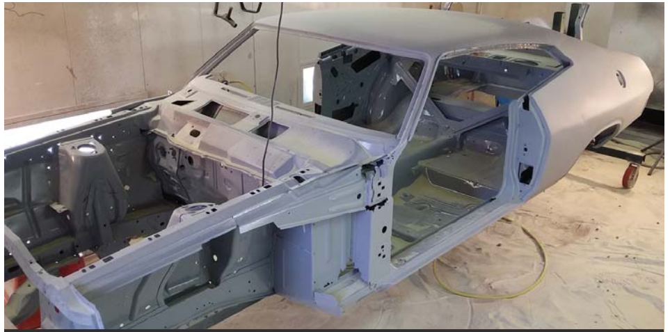
After a light media blasting, the body and panels were painted in primer before metal repair got underway.
