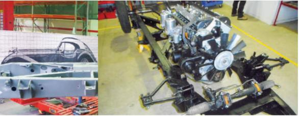
Images showing the MkV donor chassis being prepared for modification and painting; one of a series of line drawings illustrating various body style options; and the fully rebuilt 4.2 litre XK engine installed in the immaculate chassis, along with some suspension pieces and the steering.
